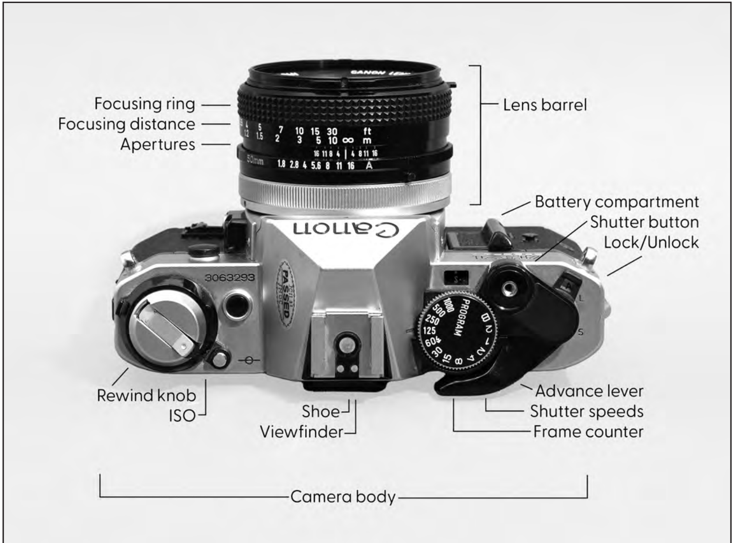
Figure 3: Diagram of 35mm camera body. Figures 4 and 5 (on right): Diagrams of mirrorless digital camera.
